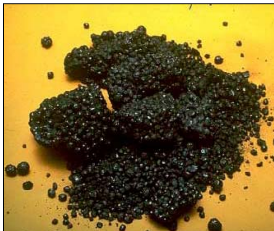
Figure 2. Shot Coke Partially Crushed
